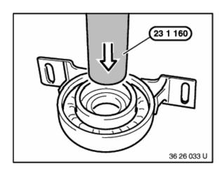
Remove centre mount, refer to 26 12 001 Press out grooved ball bearing with Special Tool 23 1 160.
