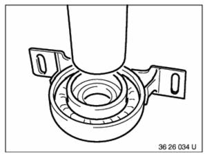
Always coat centre mount in area of ball bearing with Circolight (refer to BMW Parts Service).
